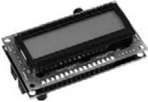
Abb. 31.1: I<sup>2</sup>C-BUS-LC-Display LCD
